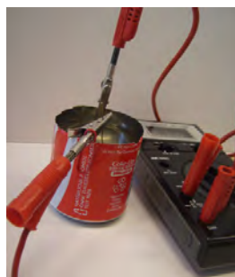
Figure 5: A simple battery
