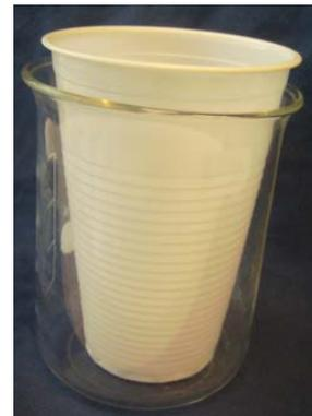
Abb. 9.3: *Low-Cost-Kalorimeter*
